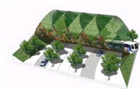
Folded meadow. The Patchwork proposal shows how an existing bridge can be transformed into an ecoduct. Green contact surface is maximized by folding the structure over itself. Illustration: KIT arkitektur
